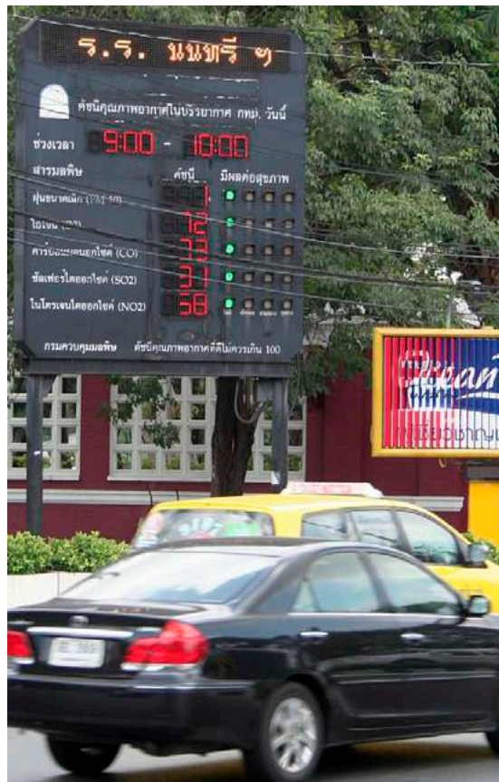
Figure 2 The number of cities in developing countries with air quality monitoring systems is increasing rapidly: An information board displaying concentrations of PM 10 , O 2 , CO, SO 2 and NO 2 in Bangkok.
